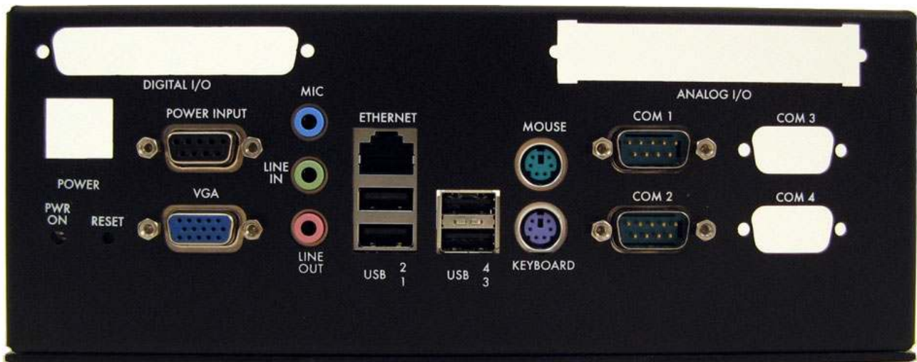
Face Plate showing 8 jack screws installed into 4 Dsub connectors
