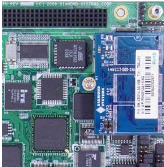
Flashdisk mounted onto Poseidon SBC
