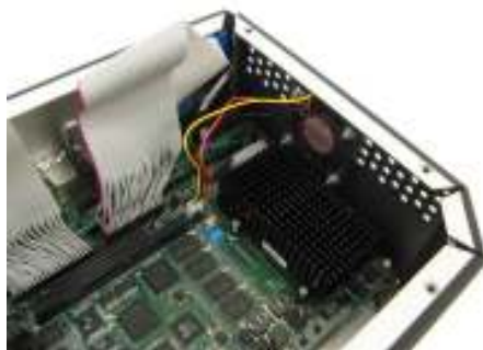
1.0GHz fan installation
