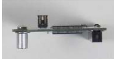
Hardware mounted onto flashdisk module
