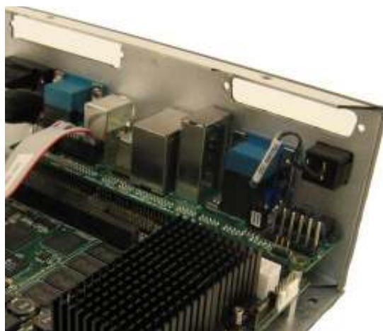
Triton Power Button (DSC cable #6981094) installed and connected to panel I/O board
