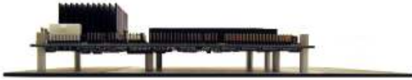
Edge view showing 7mm and 14mm spacers
