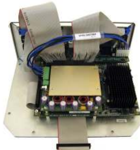
Jupiter-MM power supply attached to Poseidon
